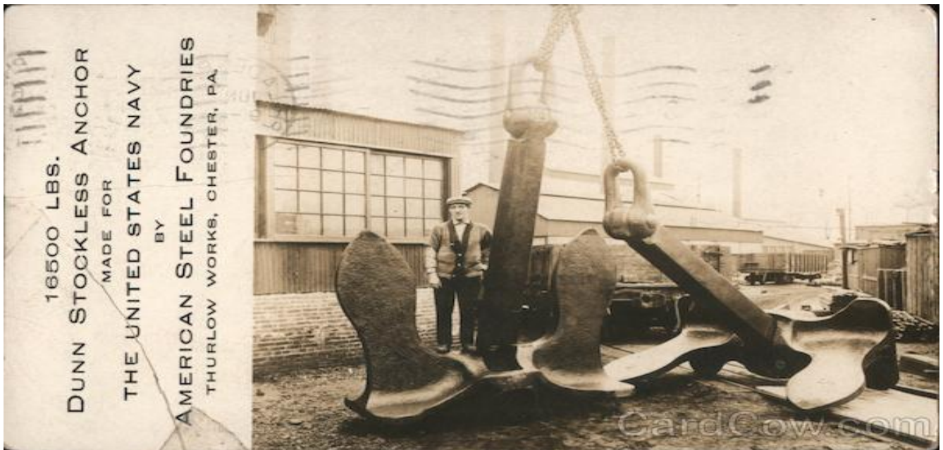
A postcard showing an example of a 16,500 pound Dunn Stockless Anchor made for the United States Navy by American Steel Foundries, a subsidiary of Thurlow Works, in Chester Pennsylvania.
